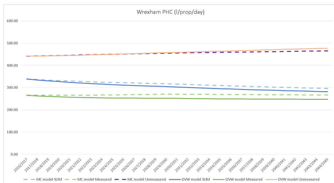
Figure B2.12 Wrexham micro-component and Hafren Dyfrdwy model comparison
