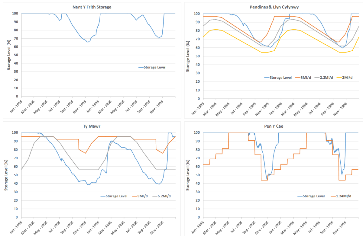
Figure 21 - Modelled reservoir storage and drought triggers for the 1995/96 drought
